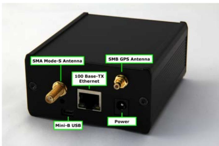
Plug the following connectors into the Radarcape:
