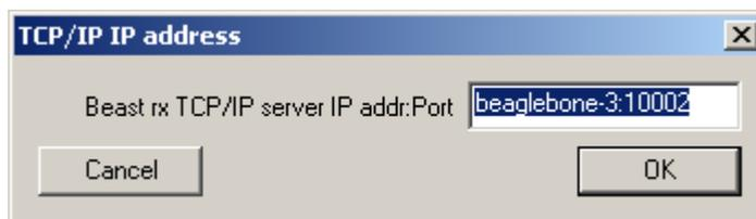
Replace *beaglebone-3* with the DNS name or IP address of your Radarcape (e.g., *radarcape.local:10002*).
