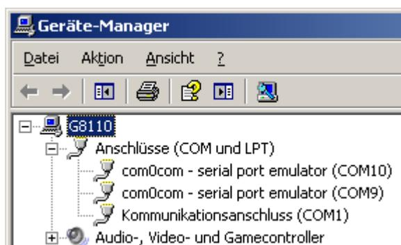
**More explanation:** Now there is a virtual link. If you have two applications that each has a serial port for data input or output, they can be linked together, one using COM9, the other one using COM10. In the COMOCOM setup it looks like this:
