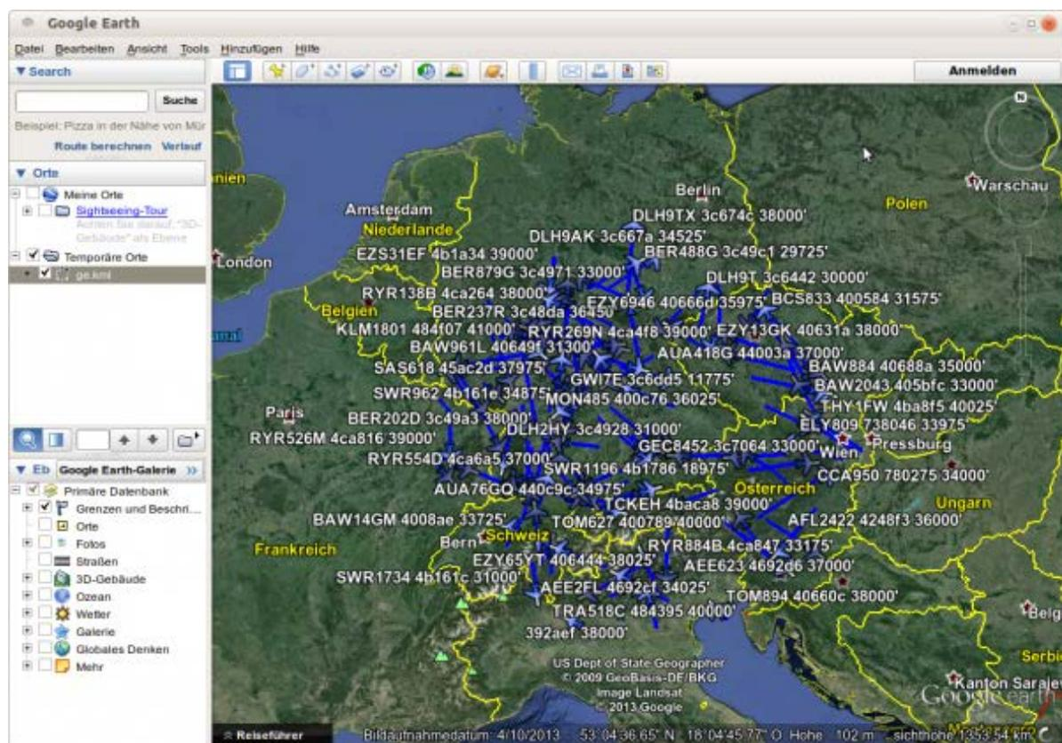
Google Earth feeded with ADS-B data from a Radarcape.
